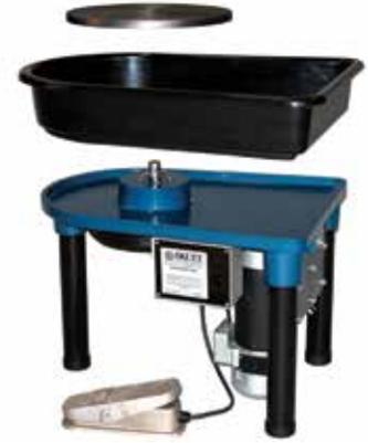
It is important to occasionally re-grease the wheel head shaft with the anti-seize grease included with your wheel. If you fail to do so, your wheel head could stick to the shaft making it difficult to remove.
