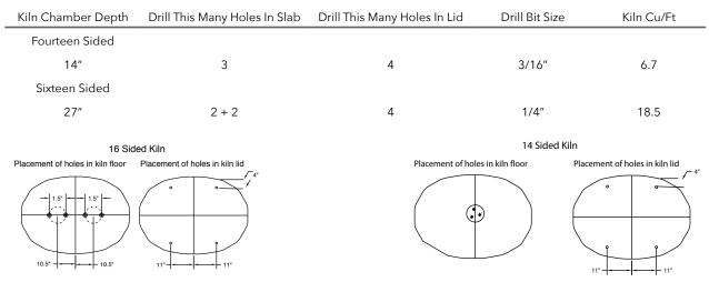
KM1627-3" kilns come with a fiber insert that sits on the slab of the kiln. If your kiln was not predrilled in the factory you will need to cut holes in these inserts to make sure the air flow is not restricted to the vent.
