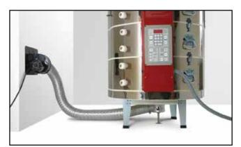
or the sound of air passage is not evident, immediately unplug the blower and check for the cause of the malfunction.
