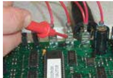
Measuring Controller Voltage
