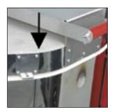
B. To line it up position the Plate overlapping the facet junction and slide it back until there is no gap between the right edge of the Pate and the lid band. Line up the bottom edge of the Catch plate flush with the bottom edge of the lid band. Attach the Plate using #103 screws.
