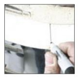
D. Align the Body Hinge Assembly so the edge is even with the top edge of the body band and the inside bend of the Body Hinges are in line with your marks. Secure with #093 screws beginning with the second column of holes in from the strut rod and working your way out. The first column of holes on each Body Hinge requires slightly longer screws so use the #756 screws.
