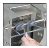
B. Slide the 5/8" upper spring retainer rod in place in the upper 5/8" holes ensuring that the upper ends of the torsion springs are behind the retainer rod. Install the hitch pins in the ends of the retainer rod.
