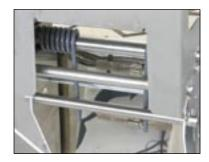
D. When the lid is carefully lowered, the torsion springs will be put in compression. Ensure that no one is standing behind the kiln when the lid is lowered until it is determined that all hinge parts are securely fastened and are working properly. Make a thorough inspection of all hinges, spring rods, etc. to ensure that nothing has worked loose.
