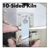
Congratulations! Your Lid Lifter Upgrade is now complete. Periodic checks should be made to the spring and hinge assembly to ensure all components are staying tight and in proper working order. A light lubricating oil may be applied to the main hinge rod if squeaking is present.
