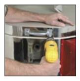
C. Remove the Lid Brace, Lid Brace Pad, and Lid Brace Guide
