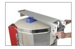
B. Line up the bottom edge of the bent flange on the front of the lid lifter arm with the bottom edge of the lid band and center the flange on the lid band using the top peep plug hole as a reference. Secure the flange to the lid band using the #103 sheet metal screws.
