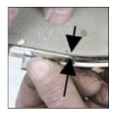
C. Position the Lid Prop Arm by placing the Prop Catch in the first notch and aligning the prop so it is perpendicular to the lid band. The Prop Arm should be able to rock back out of the closed position without catching on the Prop Catch. Secure the Prop Arm Pad with #103 screws.
