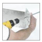
B. Stand both body hinges up on a flat surface and attach the Right Body Hinge to the other end of the strut Rod
