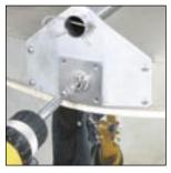
D. The Pad Eyes should be squared up with the lid band and fastened in place using the #103 sheet metal screws. The Lid Brace Pad mounts on top of the left Pad Eye. The position varies depending on the model. Check photos.
